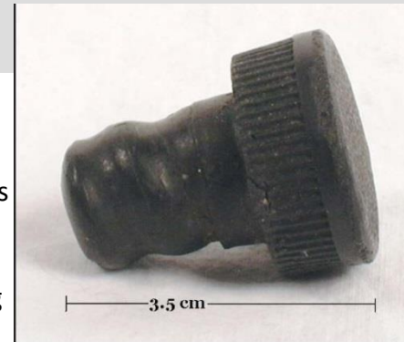
Fig. 9 Example of interior and exterior threaded plugs
