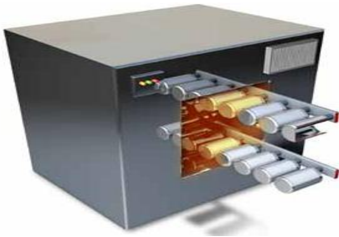
Fig. 6 Covered cans are dried in the oven.
